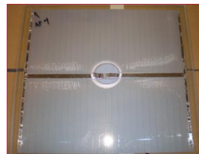
Figure 4. Typical post-nip bubble patterns for 0.2mm wide bus ribbon.
